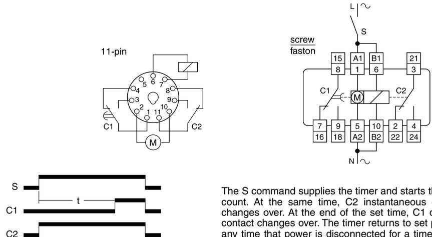
The S command supplies the timer and starts the time count. At the same time, C2 instantaneous contact changes over. At the end of the set time, C1 delayed contact changes over. The timer returns to set point at any time that power is disconnected for a time higher than 0.3 seconds.
