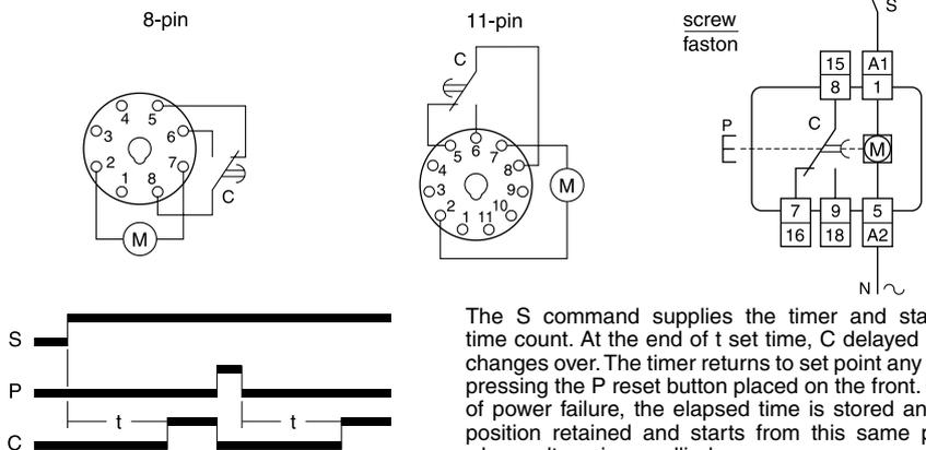
The S command supplies the timer and starts the time count. At the end of t set time, C delayed contact changes over. The timer returns to set point any time by pressing the P reset button placed on the front. In case of power failure, the elapsed time is stored and timer position retained and starts from this same position when voltage is re-applied.
