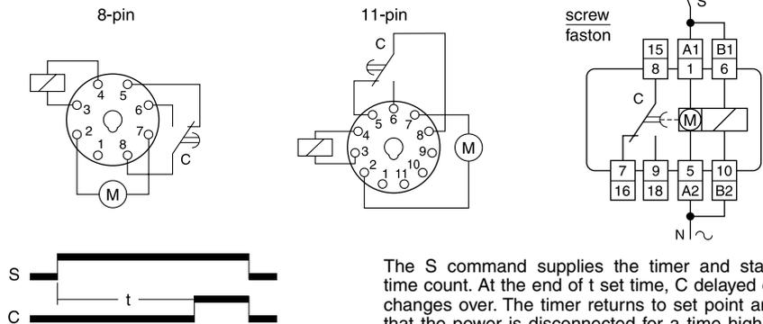
The S command supplies the timer and starts the time count. At the end of t set time, C delayed contact changes over. The timer returns to set point any time that the power is disconnected for a time higher than 0.3 seconds.
