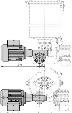
Drive with step-down gear and flange motor
