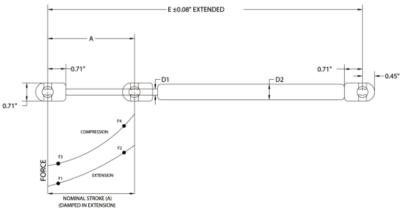
6 X 15 Carbon Steel - Fixed Force Gas Spring Forces (FI) can be factory set from 5# to 90# (22N - 400N)
