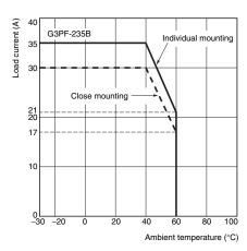
Note: The data above assumes that the Unit is mounted on a vertical surface. If it is mounted on a horizontal surface, reduce the load current shown above by 30%.
