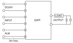
Recommended capacitor: 1  $\mu$ F, 250 VAC for the G3PF-2 $\Box$ B, and 0.5 µF, 500 VAC for the G3PF-5 B
