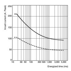
Non-repetitive input (For repetitive input, the figure will be less than the value for surge current withstand indicated by the broken line.)
