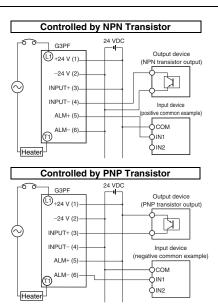
Note: With inductive loads (relay coil, etc.), connect back-current prevention diodes to both sides of the load.
