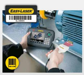
The barcode reader is used to enter the machine data before measurement is taken. After the first measurement is recorded, the adhesive barcode label is applied to the machine. Next time the machine is checked, the measurements, compensation values and tolerances can be read directly from the barcode. Simple and accurate! (\*Barcode reader is accessory.)
