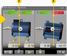
**3.** The live values reflect the adjustments made to the machine. For clarity, the adjustment is displayed both graphically and numerically. Horizontal and Vertical directions are shown at the same time.
