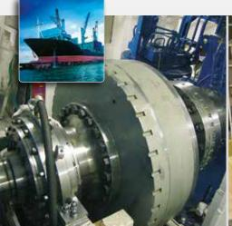
Engines, gearboxes and propeller shafts on ships are aligned using the Easy-Laser® system. Thanks to flexible brackets you can install the equipment in the most appropriate place; shaft, coupling, or flywheel.
