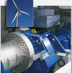
Easy-Laser® is used to align generators and gearboxes in wind turbines of a number of sizes and makes. Special brackets are available for alignment with locked rotors to increases the safety of the operator.
