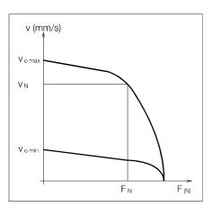
The nominal positioning force  $F_{N}$  of the actuator should exceed the break-away force  $F_{L}$  of the reel.
