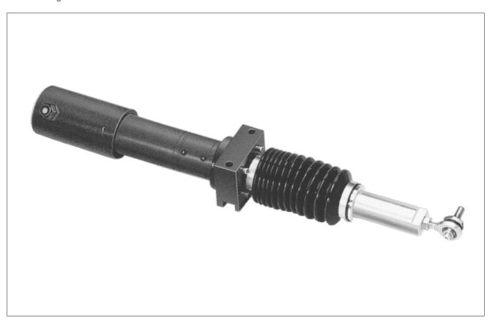
The actuator positions the reel stand axially in relation to a given web position. It consists of a shunt-wound D.C. planetary geared motor with ball screw, characterized by high efficiency and precise positioning movements.
