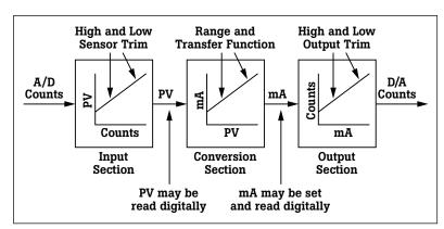
Figure A2. HART Transmitter Block Diagram.
