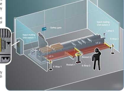
Total safety components: 2 safety light curtains - 2 restart buttons for the safety light curtains - 1 safety gate switch - 3 emergency push buttons.
