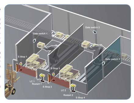
Total safety devices: 2 safety light curtains - 2 restart buttons for the safety light curtains - 3 safety gate switches - 4 emergency push buttons. Using conventional components — safety relay modules — to build up the safety circuit, it would be necessary to use at least six safety modules, wired to each other in order to perform the required functions: 2 safety relays for the light curtains - 3 safety relays for the gate switches - 1 safety relay for the emergency stop.
