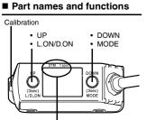
DTM: This lights up when datum calibration is performed. 1 spot: This turns off when no light enters or multiple reflections occurs.
