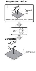
Moving target calibration (Full auto calibration. background suppression - BGS)
