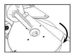
5. Remove Blade Mount Shaft.WARNING: Blade edge is very sharp.DO NOT TOUCH EDGE OF BLADE!Push the Blade Guard into the Cutter Housing just enough to clear the Blade. Remove the Blade and Blade Spacer carefully.
