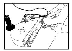
1. Loosen Rear Carriage Bolt.
