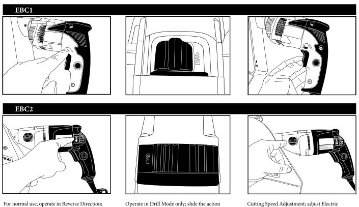
For normal use, operate in Reverse Direction; press drilling direction button for reverse direction operation.
