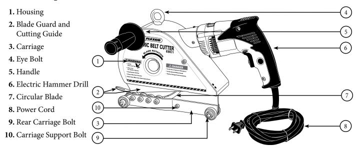
DO NOT carry tool by electric hammer drill handle. It is recommended that you place tool in carrying case for traveling extended distances.
