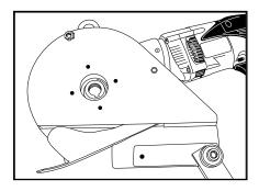
**6.** Carefully replace Blade Spacer and slide new Blade into Housing. Align keyway in Blade, Spacer, and Gearbox and insert Blade Mount Shaft. Secure Blade with Blade Mount Bolt.
