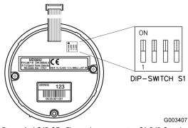
Figure 1. AC-IR-3Fq Flame detector setting S1-DIP-Switch
