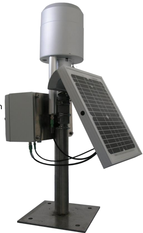
PreLOG – solar powered GPRS precipitation station
