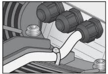
Fig. 3: Fan installed lying flat, cable routed in a U-shaped loop.
