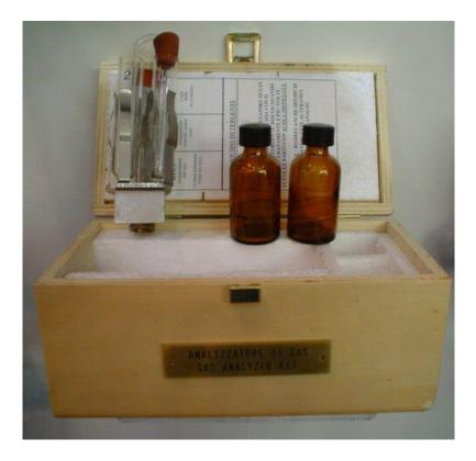
If a gas analyser kit is available it is possible to have an idea of the cause that generated the gas by checking the precipitate inside the test tube of the gas analyser.
