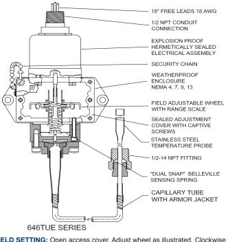
FIELD SETTING: Open access cover. Adjust wheel as illustrated. Clockwise to increase settings. Counterclockwise to decrease settings.
