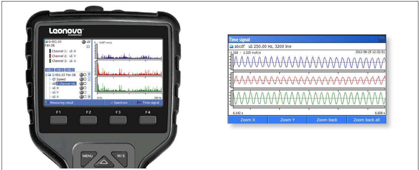
Three channel simultaneous vibration monitoring is a Leonova Diamond® function for unlimited use (DIA192) or limited use (DIA292).
