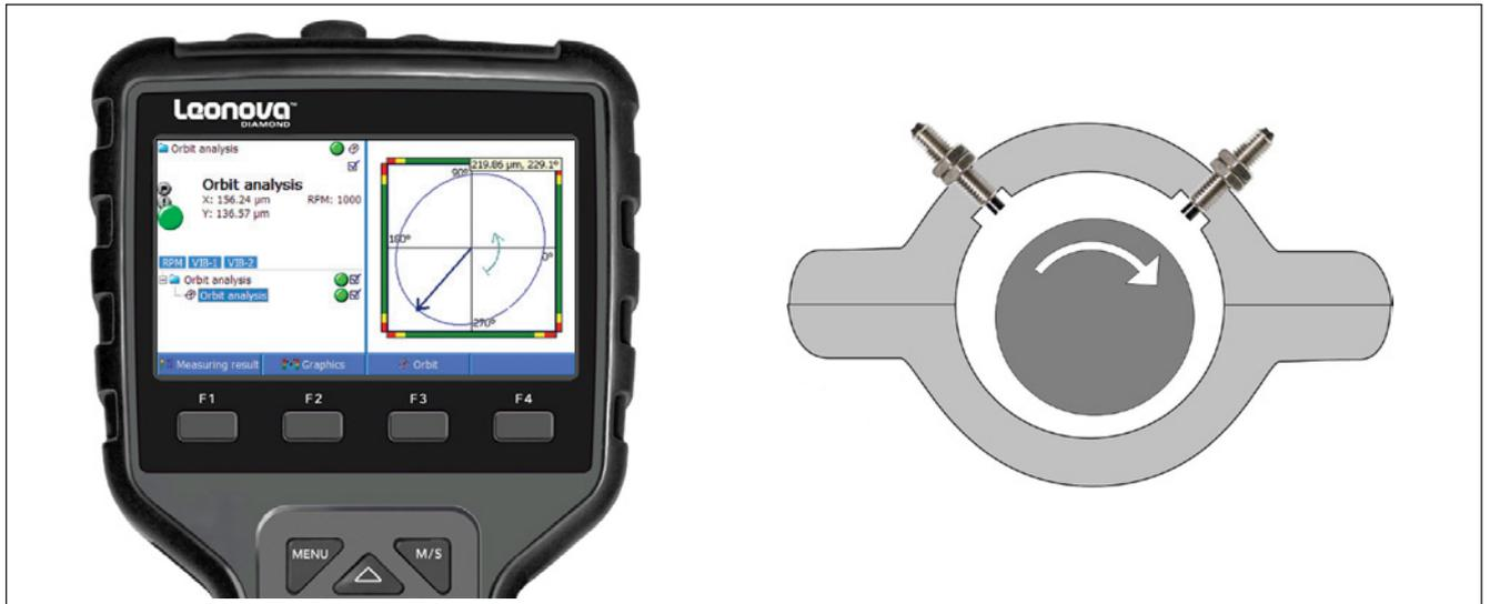
Orbit analysis and Shaft centerline plot is a vibration measurement function offered with Leonova Diamond®, for either unlimited (DIA138) or limited use (DIA238). The resulting orbit graph shows the movement of the shaft's centerline and is used to detect failures like rubs, unbalance, misalignment or oil whip on machinery with journal bearings.
