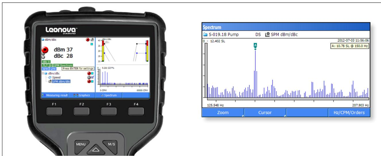
The purpose of SPM Spectrum is to verify the source of high shock pulse readings. Shocks generated by damaged bearings will typically have an occurrence pattern matching the ball pass frequency over the rotating race. Shocks from e. g. damaged gears have different patterns, while random shocks from disturbance sources have none.
