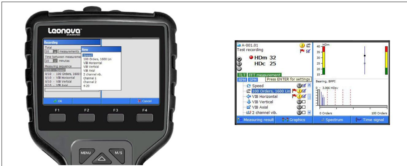
The Recording function is part of the platform, always included for unlimited use. It allows the user to measure and record measuring results over longer periods of time. The recording function is an analysis tool which can show the interaction of various condition parameters over time.
