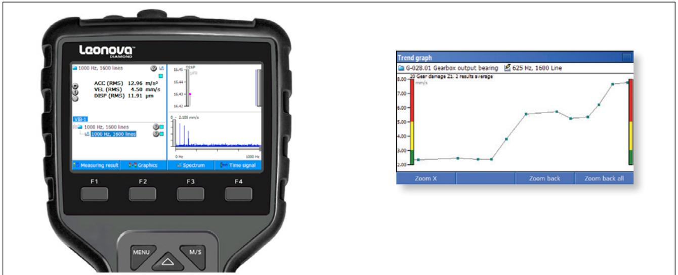
With Leonova, the EVAM method is offered as an analysing function for either limited or unlimited use. EVAM is a part of the Vibration Expert package DIA193/293 (TD-365).
