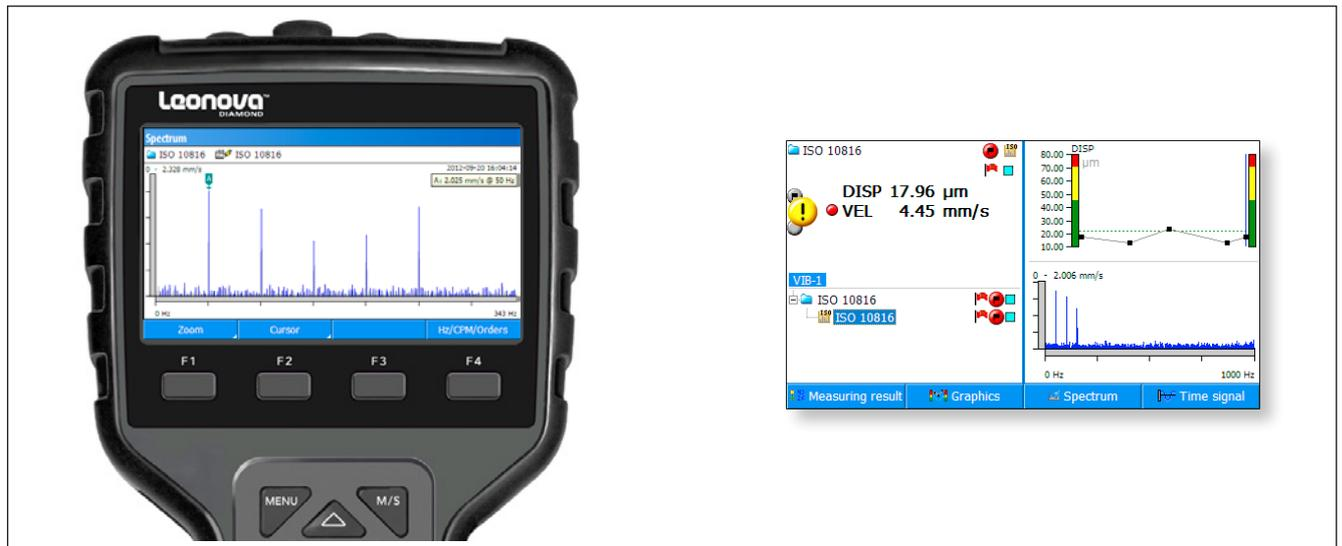
Broadband vibration measurement is the most widely used and cost-efficient method for the diagnosis of general machine condition.
