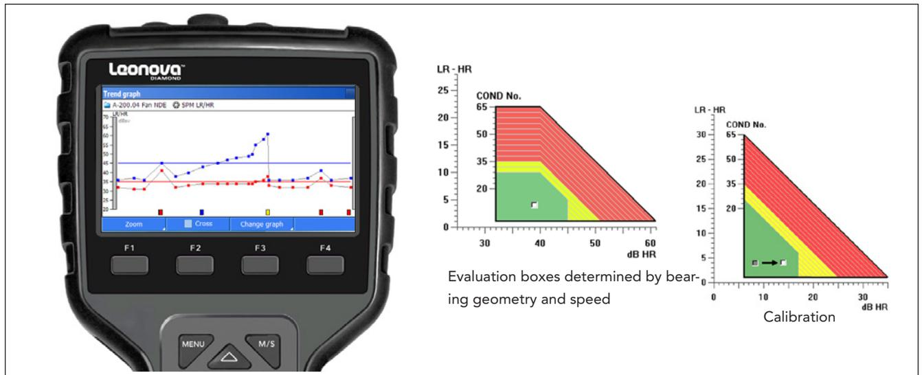
The LR/HR method was developed from the original Shock Pulse Method for condition diagnosis of rolling element bearings. It allows a precision analysis of oil film condition in the rolling interface and contains computation models for finding the optimal lubricant. Poor lubrication is the root cause of most bearing failures.
