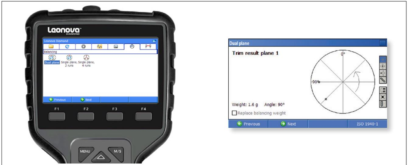
Single and dual plane balancing are optional Leonova functions for either limited or unlimited use. In case of limited use, credits are deducted for each vibration measurement.
