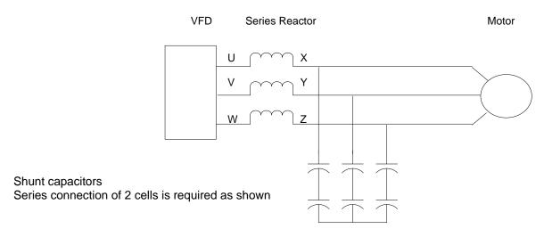
NOTE: All 690V SWF filters require series connection of capacitors in each phase as shown.
