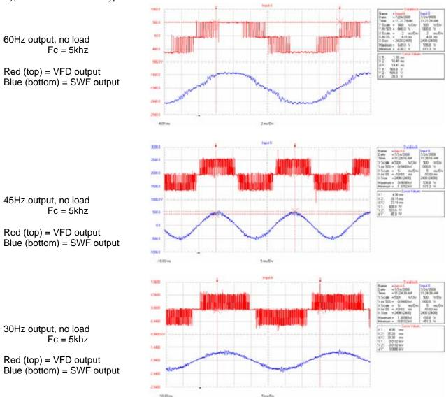
Typical results for 5KHZ type sine wave filter:
