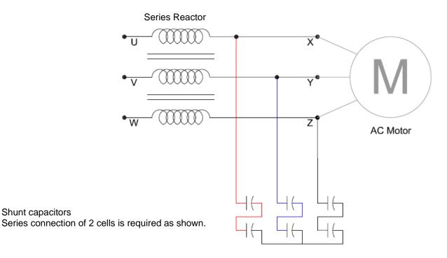
When our (WH-xxxx) wiring harness kits are used, the wires supplied are Red, Blue and White.
